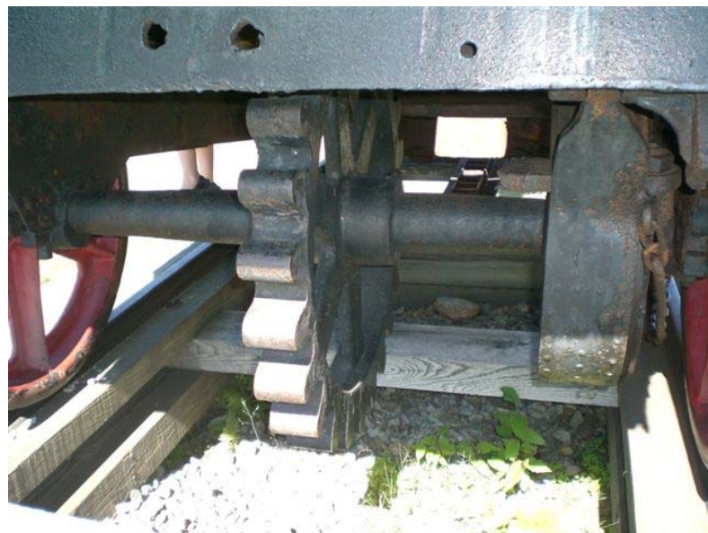
The cog on the locomotive that engages the rack to propel the train up the mountain.
